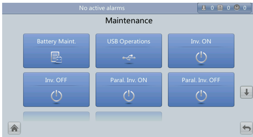
Figure 4-53 Maintenance Screen (parallel system)
